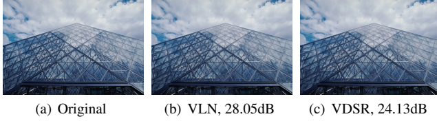
Fig. 3. Deep learning-based image interpolation and their PSNR results.
